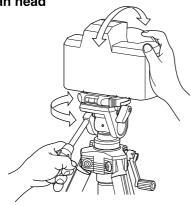
When you unlock the handle, your camera is free to move up and down. When the pan & tilt handle is unlocked, you can pan & tilt simultaneously.
