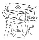
Remove the Quick Release Platform turning the Lock lever. In this case, please do not put the Lock Lever back by force as it has been stood by the Stopper.
