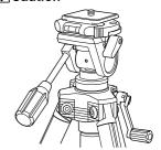
Prevent accidental equipment fall, or tripod tipping over, by making sure all levers, knobs, and handles on the tripod are securely tightened, and that all three legsare opened all the way.
