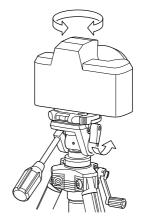
When you unlock the Camera platform locking knob, raise the knob it to the vertical "release" position. The camera can be free to rotate.
