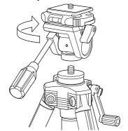
Set the head on the tripod's threaded post. Turn clockwise until it comes to a stop
