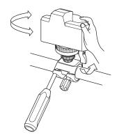
The camera platform can be rotate 360 degree when the camera platform locking lever is unlocked.
