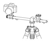
When the arm is stretched to the one direction, a tripod can loose the balance easily and may tip over. To prevent this, set your camera close to the body.
