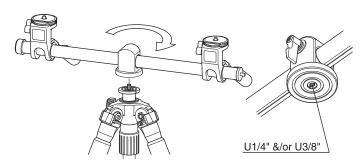
Set the head on the tripod's threaded post. Turn clockwise until it comes to a stop.
