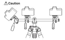
The tripod may be easily tipped over when the overall balance is broken.
