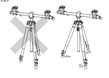
To prevent accidental equipment fall or tripod tipping over, making sure all levers, knobs and handles on the tripod are securely tightened. And all of the three legs are opened all the way.
