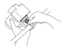
Hold the camera firmly when the camera mounting screw turn to engage the threads.
