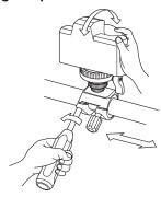
The pan head is tilted and moved right or left when the pan handle is unlocked. The friction knob controls frictions for the both of tilting and sliding.
