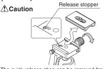
The quick release shoe can be removed from the top when the shoe locking knob is loosened fully, when the shoe locking knob is loosened fully, the release stopper mechanism does not work. Be careful not to come off the quick release shoe accidentally.
