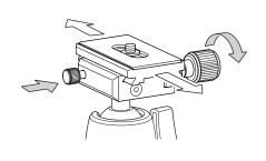
Tighten the ball fixing lever and pan fixing knob. When a tripod mounting screw is U3/8", screw in the double screw adaptor.
