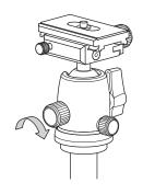
A friction is adjusted by the tension adjustment knob only when the ball fixing lever is loosened.
