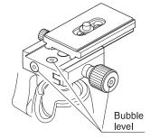
Adjust the bubble level to fit into center. The bubble level is a rough criterion. It is not accurate as a leveler on a camera.
