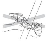
Do not use an optional clamp head for a carbon fiber monopod. The pipe may be damaged.
