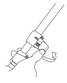
Flip up the leg lock lever to extend or shorten any of the individual leg sections to the desired length and close the leg lock lever.
