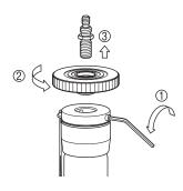
When the Camera mounting is converted to U3/8" screw, remove the fixing screw with an allen wrench.
