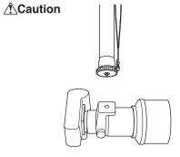
Hold the camera firmly, and screw the monopod into tripod socket.
