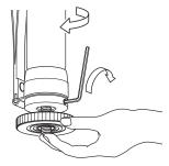
When the Camera platform is attached, make the monopod upside down and turn the monopod body clockwise while holding the Camera platform and the Camera mounting screw.
