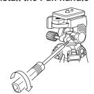
Install the Pan handle to the appropriate position on the Pan head.
