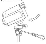
With your camera mounted on the Quick release, move the Quick release lock fully to the right and place your camera into position.
