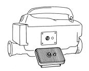
Mount your Camera to the Quick Release Platform by inserting the threaded Camera Post into the Tripod Mounting Socket of your camera. Raise the Wing Nut on the Camera Post and turn it counterclockwise until your camera is locked in position. (Make sure camera is locked firmly into position but do not overtighten.)
