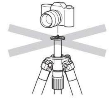
Do not attach a camera directly to the Pan head attachment screw. This may damage both your camera and tripod.
