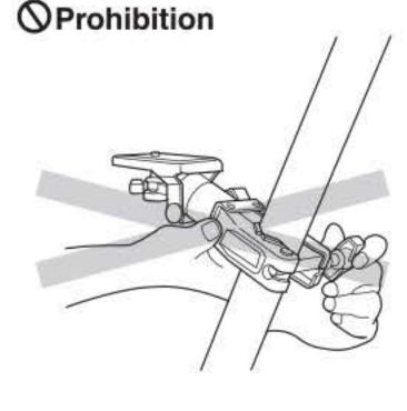
Do not use an optional clamp head for a carbon fiber tripod. The pipe may be damaged.
