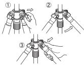
To change the angle of each leg, close the leg slightly, and then pull the leg angle adjustment lock out. There is a choice of two other angle positions. After choosing the desired leg angle, securely push in the adjustment lock.
