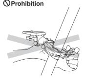
Do not use an optional clamp head for a carbon fiber tripod. The pipe may be damaged.
