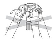
Do not turn the center column stopper while pulling out the center column.
