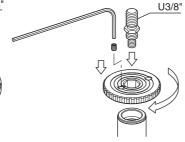
Flip the panhead attachment screw and put back to the center coumn plate. Screw in the center column plate and the panhead attachment screw. Tighten the fixing screw to avoid the rotating the center column plate while in use.
