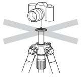
Do not attach a camera directly to the Pan head attachment screw. This may damage both your camera and tripod.
