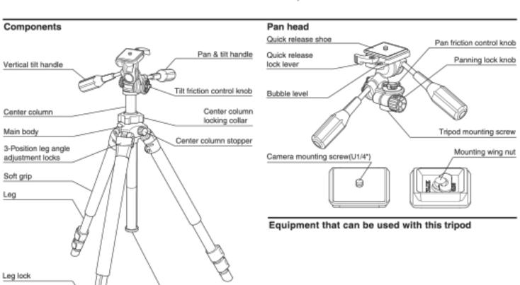
This product has been designed to handle an equipment weighing under 5 kg (11 lbs). Do not overload.
