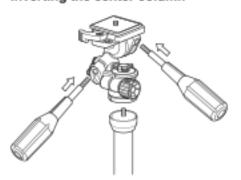
Always remove the pan head first before replacing the center column.
