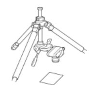
By inverting the center column, it is possible to do copy, and close up work.
