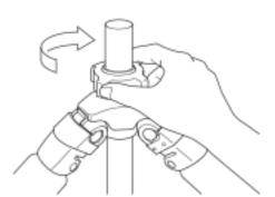
Insert the center column from lower side of main body, and tighten the locking collar and the center column stopper.
