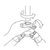
Loosen the center column stopper and the locking collar, and then pull out the center column.
