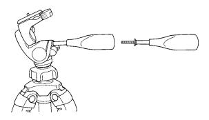
Remove the Vertical tilt handle from the Pan head, and screw into the back of the Pan & Tilt handle.
