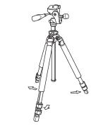
Be sure to open all three legs completely in order to prevent camera shakes, or accidental tip overs caused by unstableness.
