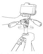
Hold onto the Pan head with one hand, and loosen the Center column stopper and the Center column locking collar with the other hand. Raise or lower Pan head to desired height, and while maintaining a hold of the Pan head, tighten the Locking collar and the stopper.
