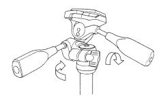
Set the new head, or accessory on the tripod's threaded post, and turn clockwise until it comes to a stop. Tighten the Panning lock knob and turn clockwise slightly more.
