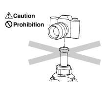
Do not attach camera directly to the threaded post of the Center column.
