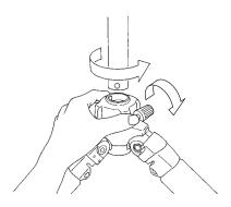
Loosen the Center column stopper and the Locking collar, and then pull out the Center col-
