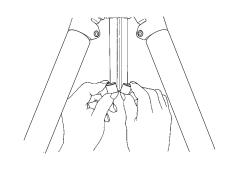
Remove the Rubber stopper from the bottom of the column.
