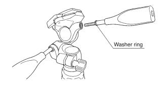
Check to see that there is a Washer ring on the shaft of the Vertical tilt handle, and then insert the shaft into the threaded hole located on the right side of the Pan head. Screw handle all the way in until secure.
