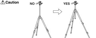
To avoid unnecessary camera vibrations, try to keep the Center column height to a minimum.
