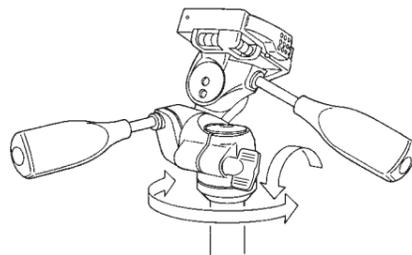
Loosen the Panning lock knob, and the head will rotate along the horizontal direction.
