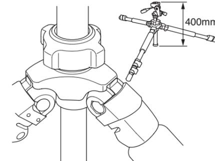
After choosing the desired leg angle, securely push in the Adjustment lock.
