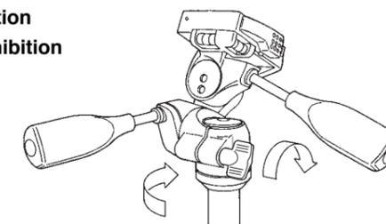
Set the new head, or accessory on the tripod's threaded post, and turn clockwise until it comes to a stop. Tighten the Panning lock knob and turn clockwise slightly more. Do not attach camera directly to the threaded post of the Center column. This can damage both camera and tripod.
