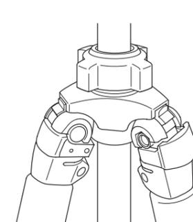
To change the angle of each leg, close the leg slightly, and then pull the Leg angle adjustment lock out. There is a choice of two other angle positions.
