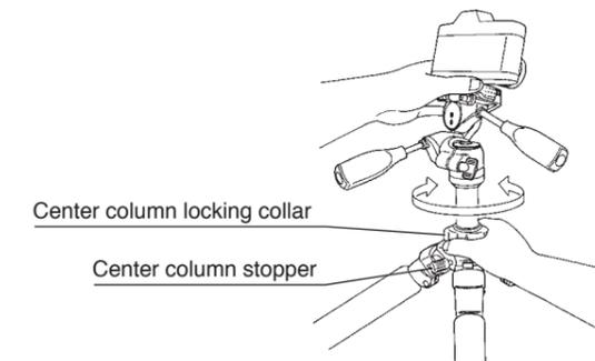
Hold onto the Pan head with one hand, and loosen the Center column stopper and the Center column locking collar with the other hand. Raise or lower Pan head to desired height, and while maintaining a hold of the Pan head, tighten the Locking collar and the stopper.
