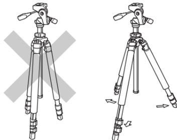
Be sure to open all three legs completely in order to prevent camera shakes, or accidental tip overs caused by unsteadiness.
