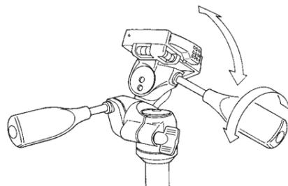
Loosen the Vertical tilt handle, and the level can be adjusted.
