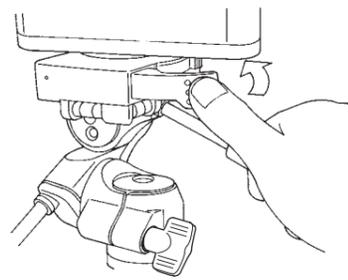
Fix the Quick shoe at a desired position by closing the Locking lever.
