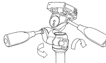
Use the following instructions if you wish to change heads, or attach accessories. First, lock the Panning lock knob, then grasp the pan, or Vertical tilt handle and turn the head, counter-clockwise to loosen.
