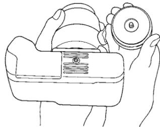
Screw quick shoe on to camera, and insert back into the Camera platform. Please DO NOT over tight your Quick release platform.
