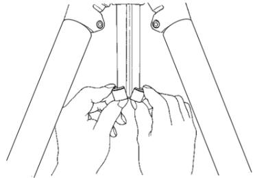
Remove the Rubber stopper from the Bottom of the Center column.
