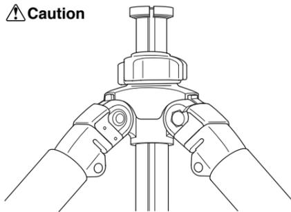
Make sure to re-attach the Rubber stopper, in order to prevent the Center column from falling out.
