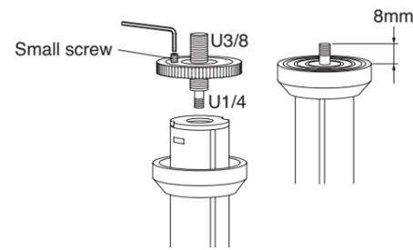
4. Loosen the Pan head fixing screw and pull it out. Then, screw it in again after reversing top and bottom.
