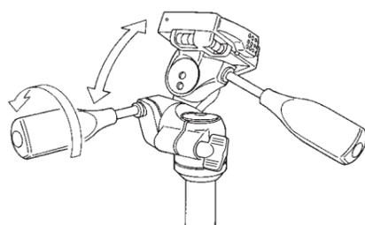
Loosen the Pan & Tilt handle, and the head will tilt back and forth.
