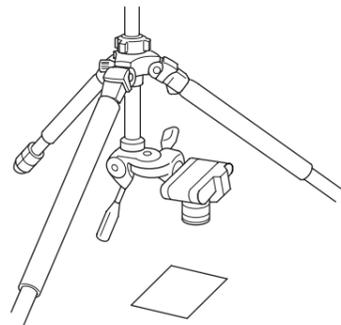
By inverting the Center column, it is possible to do copy, and close up work. Follow the same procedures in order to replace with optional Short center column.
