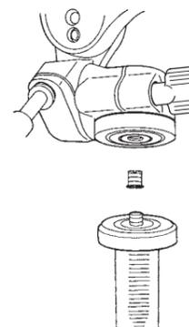
When attaching the Pan head to a tripod with a small thread(U1/4) use the optional small thread adapter.
