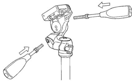
Attach the two Pan handles to the Pan head, by inserting the shorter handle to the left, and the longer horizontal tilt handle to the right. Do not reverse.
