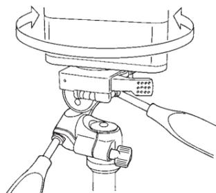
Correctly installed you will hear a "click", and the Quick shoe will rotate 360°.
