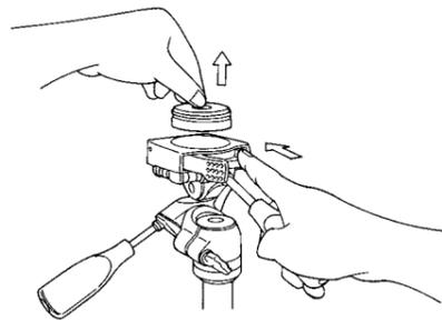
Remove Quick release platform by opening the Locking lever and then pressing the Release button.
