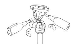
Set the new head, or accessory on the tripod's threaded post, and turn clockwise until it comes to a stop. tighten the panning lock knob and turn clockwise slightly more.
