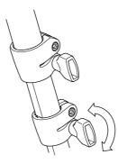
To extend, or shorten a leg, loosen the leg lock knob by turning it counter clockwise. Turn knob clockwise to tighten, at the desired height. Do not over tighten the leg lock knob, as this may damage the leg tube.
