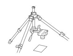
Always remove the pan head when replacing the center column.
