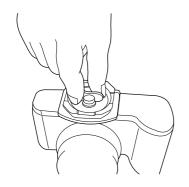
Align the length of the quick release shoe along the base of the camera body, and securely tighten the mounting wing nut.
