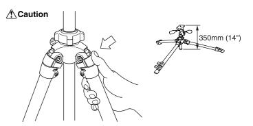
After choosing the desired leg angle, securely push in the adjustment lock. By using the optional short center column, you can obtain the lowest camera height of 350 mm (14").
