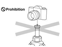
Do not attach camera directly to the threaded post of the center column.
