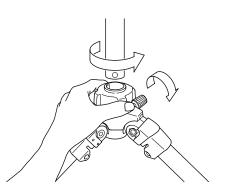
Insert the center column from the lower side of main body, and tighten the Locking collar and the center column stopper.
