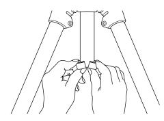
Loosen the center column stopper and the Locking collar, and then pull out the center column.
