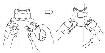
To change the angle of each leg, close the leg slightly, and then pull the leg angle adjustment lock out. There is a choice of two other angle positions.
