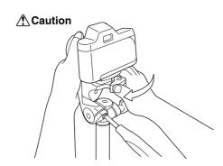
When attaching the camera to the pan head, check to make sure that the quick release shoe is engaged in the catch of the pan head before locking the lever.
