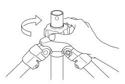
Make sure to re-attach the rubber stopper, in order to prevent the center column from falling out.
