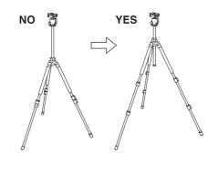
To avoid unnecessary camera vibrations, try to keep the center column height to a minimum. Also use the larger legs first when extending the legs.
