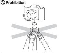
Do not attach a camera directly to the pan head attachment screw.
