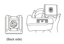
Screw the camera mounting screw on the tripod attachment screw of your camera and fix firmly.
