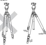
To prevent accidental equipment fall or tripod tipping over, making sure all levers, knobs and handles on the tripod are securely tightened. And all of the three legs are opened all the way.
