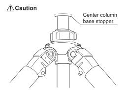
Always be sure to return the center column base stopper back on the center column. This prevents the center column pulled out accidentally.
