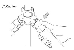
After choosing the desired leg angle, securely push in the adjustment lock
