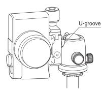
To set vertical camera position, place the platform into U-groove.
