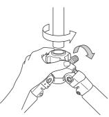
Loosen the center column stopper and the locking collar, and then pull out the center column.
