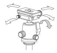
The platform can be moved freely while ball fixing lever is loosened.
