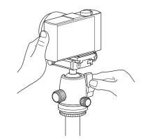
To loosen the ball fixing lever with a camera on can result an unexpected fall. Hold a camera firmly until the ball fixing lever is tightened.
