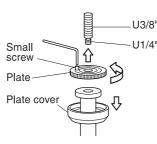
The pan head attachment screw is reversible for either large thread (U3/8") or small thread (U1/4").
