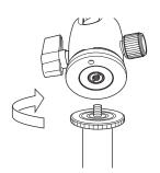
Fasten the ball fixing lever and screw into a tripod mounting screw.
