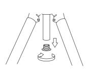
Remove the center column base stopper from the bottom of the center column.
