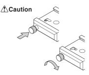
To make the release stopper ineffective, turn the safety release knob while pushing.
