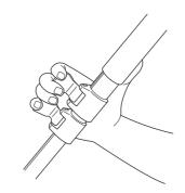
Flip up the leg lock lever to extend or shorten any of the individual leg sections to the desired length. Press the leg lock lever flush against the leg to lock.
