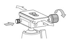
Loosen the shoe locking knob. Slide out the guick release shoe from the platform while pushing the safety release knob.
