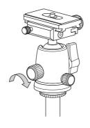
A friction is adjusted by the tension adjustment knob only when the ball fixing lever is loosened.
