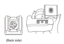
Screw the camera mounting screw on the tripod attachment screw of your camera and fix firmly.
