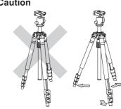
To prevent accidental equipment fall or tripod tipping over, making sure all levers, knobs and handles on the tripod are securely tightened. And all of the three legs are opened all the way.
