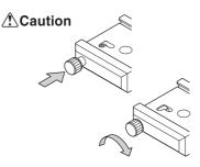
To make the release stopper ineffective, turn the safety release knob while pushing. When the release stopper is ineffective, be careful
