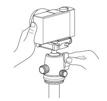
To loosen the ball fixing lever with a camera on can result an unexpected fall. Hold a camera firmly until the ball fixing lever is tightened.
