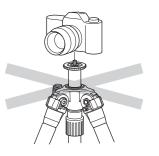
Do not attach a camera directly to the pan head attachment screw.
