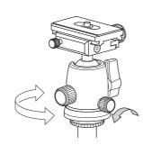
When the pan fixing knob is loosened, the tripod head is rotated horizontally.
