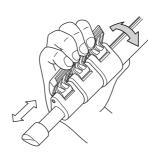
Flip up the leg lock lever to extend or shorten any of the individual leg sections to the desired length and press the leg lock lever flush against the leg to lock.
