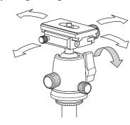
The platform can be moved freely while ball fixing lever is loosened.
