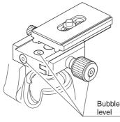
Adjust the bubble level to fit into center. The bubble level is a rough criterion. It is not accurate as a leveler on a camera.
