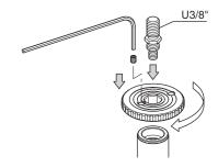
Flip the pan head attachment screw and put back to the center column plate. Screw in the center column plate and the pan head attachment screw. Tighten the fixing screw to avoid the rotating the center column plate while in use.
