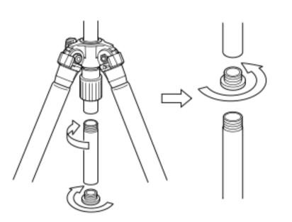
Remove the center column base stopper and then, remove the lower part of center column.
