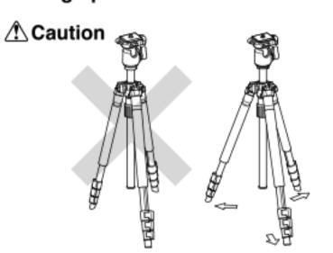
To prevent accidental equipment fall or tripod tipping over, making sure all levers, knobs and handles on the tripod are securely tightened.
