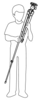
It is easier to extend the tripod legs if you turn the leg-tips to the foot, while leaving legs close.
