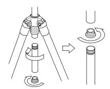
Remove the Center Column Base Stopper and then, remove the Lower part of
