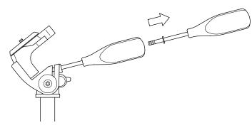
Remove the Vertical Tilt Handle from the back of the Pan & Tilt Handle where it is stored.
