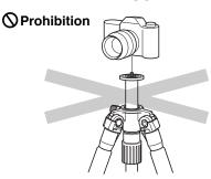
Do not attach camera directly to the threaded post of the Center Column.
