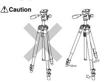
Prevent accidental equipment fall, or tripod tipping over, by making sure all levers, knobs, and handles on the tripod are securely tightened, and that all three legs are opened all the way.
