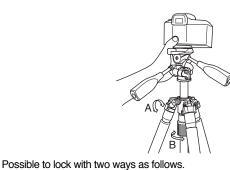
A. by Screw-type center column stopper. B. by Twist-type center column locking nut. Screw-type center column stopper will be steady, while sideslipping. Twist-type center column locking nut will be no sideslipping, but not enough to stop sometimes.
