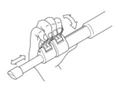
Flip up the leg lock lever to extend or shorten any of the individual leg sections to the desired length and press the leg lock lever flush against the leg to lock.
