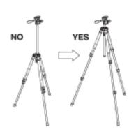
To avoid unnecessary camera vibrations, try to keep the center column
