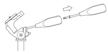
Remove the Vertical Tilt Handle from the back of the Pan & Tilt Handle where it is stored.
