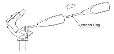
Remove the Vertical Tilt Handle from the Pan Head, and screw into the back of the Pan & Tilt Handle.
