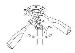
Loosen the Panning Lock Knob, and the head will rotate along the horizontal direction.
