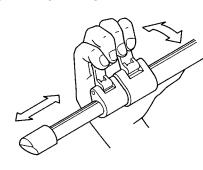
Flip up the Leg Lock Lever to extend or shorten any of the individual leg sections to the desired length, and press the Leg Lock Lever flush against the Leg to lock.
