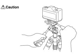
When loosening either the Pan & Tilt Handle, or the Vertical Tilt Handle, take precaution by keeping a firm grip on the handle until the Pan Head is locked down.
