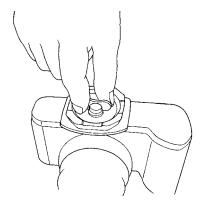
Align the length of the Platform along the base of the camera body, and securely tighten the Mounting Wing Nut.
