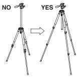
To avoid unnecessary camera vibrations, try to keep the Center Column height to a minimum
