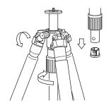
Remove the Rubber Stopper from the Bottom of the Center Column. Loosen the Center Column Stopper and the Locking Collar, and then pull out the Center Column.
