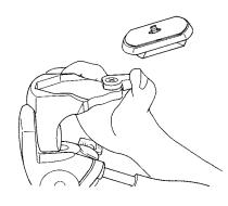
To remove the Quick Release Platform from the Pan Head, turn Quick Release Lock Lever and lift out Platform from its back.
