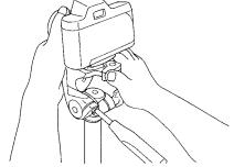
When attaching the camera to the Pan Head, check to make sure that the Quick Release Platform is engaged in the catch of the Pan Head before locking the lever.
