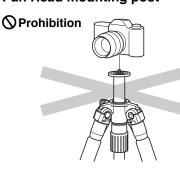
Do not attach camera directly to the threaded post of the Center Column.
