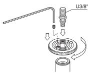
Flip the panhead attachment screw and put back to the center coumn plate. Screw in the center column plate and the panhead attachment screw. Tighten the fixing screw to avoid the rotating the center column plate while
