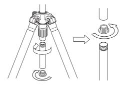
Remove the center column base stopper. Then remove the lower part of center column
