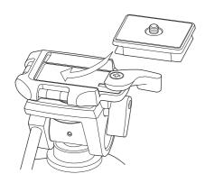
To attach the quick release shoe, slide into quick release shoe slantways. If will be closed automatically after attaching.
