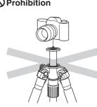
Do not attach camera directly to the threaded post of the center column. This may damage both camera and tripod.
