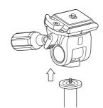
Remove the center column base stopper from the bottom of the center column.
