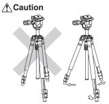
To prevent accidental equipment fall or tripod tipping over making sure all levers, knobs and handles on the tripod are securely tightened, and that all three legs are opened all the way.
