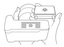
Insert the camera mounting screw on the quick release shoe in the place of the tripod attachment screw of your camera.
