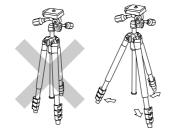
To prevent accidental equipment fall or tripod tipping over making sure all levers, knobs and handles on the tripod are securely tightened, and that all three legs are opened all the way.
