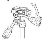
When you unlock the Vertical tilt handle, your camera is free to move up and down.
