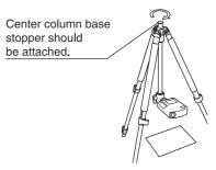
Insert a Center column from the bottom. Tighten a Center column stopper and Center column locking nut firmly.
