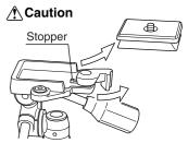
To remove the Quick release plate, turn the Quick release plate locking lever. In this case do not put the lock lever back by force as it has been stood by the stopper.
