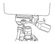
To attach the plate, slide into Quick release plate slantways. If will be closed automatically after attaching.
