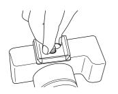
Insert the Camera mounting screw on the Quick release plate in the place of the tripod attachment screw of your camera.
