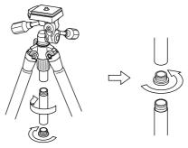
Remove the Center column base stopper. Then remove the Lower part of Center column. Put the Center column base stopper in to the Upper part of Center column.
