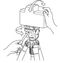
When you unlock the handle, your camera is free to move up and down. When the pan & tilt handle is unlocked, you can pan & tilt simultaneously.
