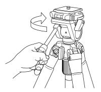
Set the new head or accessory on the tripod's threaded post. Turn clockwise until it comes to a stop.
