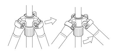
To change the angle of each leg, close the leg slightly. Then pull the 3-position leg angle adjustment locks. There is a choice of two other angle positions.
