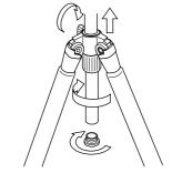
It can be used for digital copy/or close-up photography when a Center column is inserted from the bottom.
