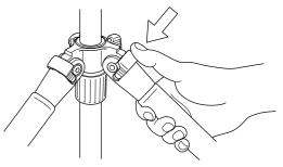
After choosing the desired leg angle, securely push the Adjustment lock.
