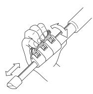
Flip up the Leg lock lever to extend or shorten any of the individual leg sections to the desired length. Press the leg lock lever flush against the leg to lock.
