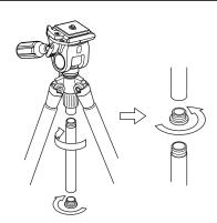
Remove the Center column base stopper. Then remove the Lower part of Center column. Put the Center column base stopper in to the Upper part of Center column
