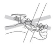
Do not use an optional Clamp head for a carbon fiber tripod. The pipe may be damaged.
