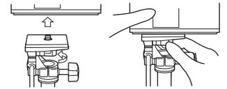
Attach camera by rotating Camera Mounting Screw counterclockwise until camera is firmly seated on tripod platform.
