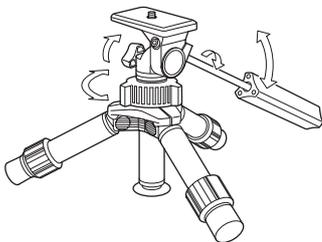
Loosen the Pan & Tilt Handle to tilting, the Panning Lock Knob to panning and move the camera into the desired shooting position. Turn the Handle and the Knob clockwise to lock the camera in position.
