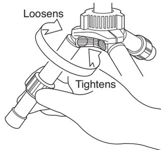
To extend any leg, turn the Leg Lock Nut one half turn counterclockwise.
