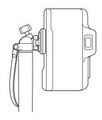
Then turn the Camera platform to tilt 90° from horizontal to vertical by using Tilt lock knob. When using vertical position, ensure the camera is securely tightened to the Camera platform.
