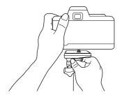
Hold the camera firmly, and turn the camera mounting screw until the camera securely tightened.
