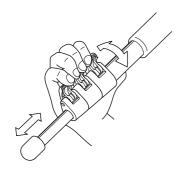
To extend the leg sections, open the Leg lock lever and extend the Slim-Pod  ${\rm I\!I}$  to the approximate desired height. Close the Leg lock lever by pressing them down.
