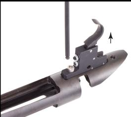
2) Using an Allen Key unscrew the trigger fixing screw and remove the trigger from the action.
