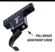
Your TriggerTech trigger is set near the middle of the advertised pull weight range and can be adjusted in increments. To adjust pull weight, insert the supplied 5/64" Allen wrench into the set screw located at the bottom of your trigger. To increase pull weight, rotate the set screw clockwise. Pull weight can vary between actions.
