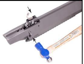
4a) Insert the trigger assembly, ensuring that the holes are aligned and gently tap the front trigger pin in.
