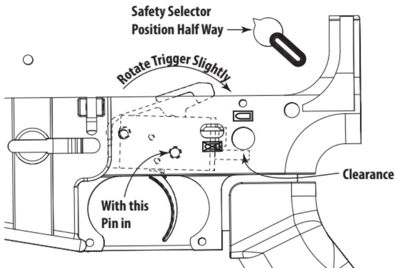
4a) With only the rear pin in the trigger, rotate the trigger assembly as shown, so the safety will not interfere when being inserted.
