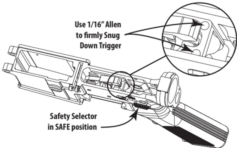
**IMPORTANT:** It is **CRITICAL** that you firmly, and **PROPERLY**, tighten **BOTH** Snug Down screws prior to re-assembling your firearm.
