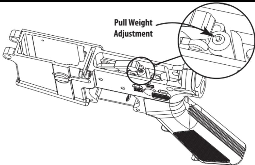
**IMPORTANT:** Some TriggerTech models allow you to adjust your trigger pull weight. The set screw is located towards the rear-center of the trigger and is set near the middle of the advertised pull weight range. To adjust pull weight, insert the supplied 5/64" Allen wrench. To increase pull weight, turn the set screw clockwise.
