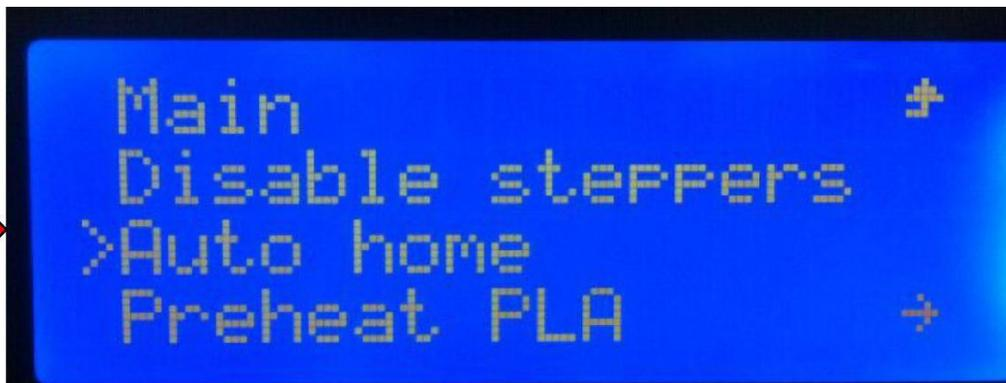
**Select "AUTO HOME" instruction, the axes will move to the zero position (bottom left corner), after the hit limit switch stops, meaning the direction is correct.**
