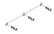
3 Install screws to fix product to wall.
