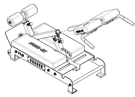
2. Unlock the incline adjustment part and insert the top part with the cushions on to the other hole.
