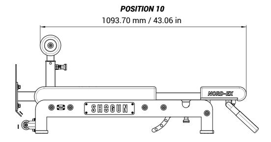
THE NORD-EX LENGTH CAN BE ADJUSTED TO FIT TALLER USERS, USE HOLE POSITIONS 8-10 TO ADJUST THE LENGTH.
