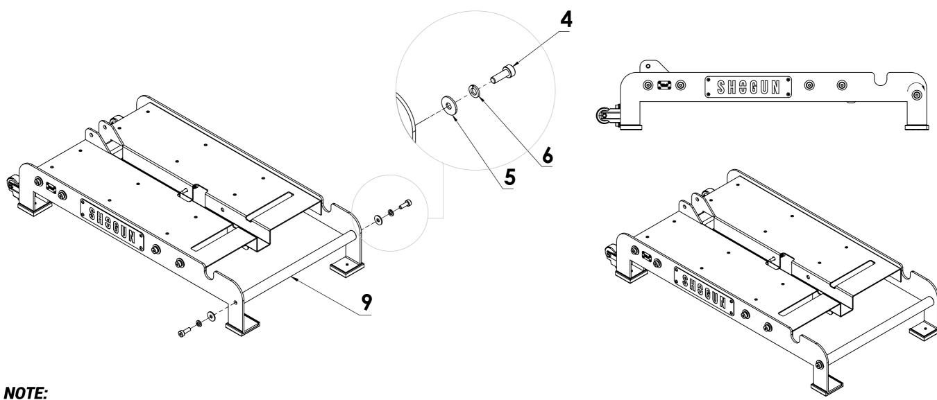
You might need to loosen up some of the screws on the side panels to comfortably insert the handle tube.
