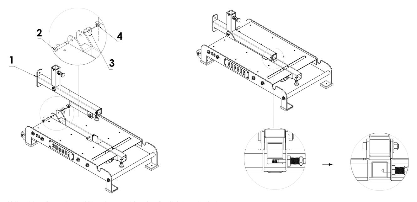
Ensure it's fully tightened to avoid any wobbliness issues. Pull the safety pin to lock the product in place.
