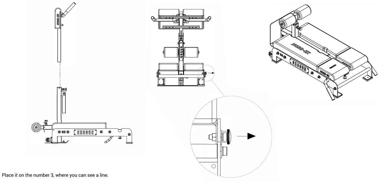
This is the default position, carefully lower the entire back extension, and lock it using the safety pin.
