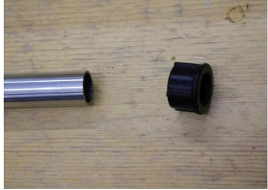
Photo 8: Silicone top cap and top end of outer siphon tube
