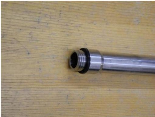
Photo 6: Silicone gasket installed
