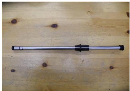
Photo 10: Completed siphon body assembly
