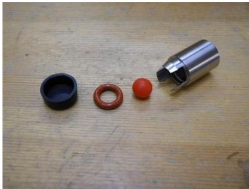
Photo 1: Check valve parts:
