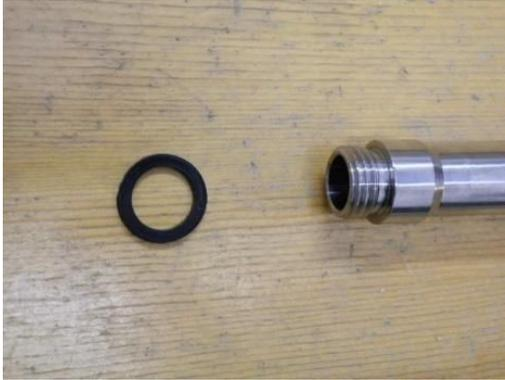
Photo 5: Silicone gasket and threaded end of outer siphon tube
