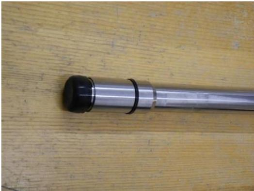
Photo 7: Check valve assembly installed on outer siphon tube
