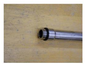
Photo 6: Silicone gasket installed
