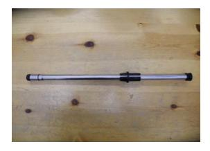
Photo 10: Completed siphon body assembly
