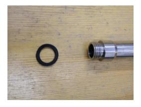
Photo 5: Silicone gasket and threaded end of outer siphon tube
