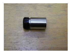
Photo 4: Completed check valve assembly
