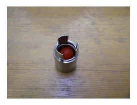
Photo 2: Check valve ball in place in check valve body
