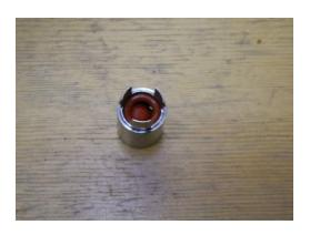
Photo 3: O-ring in place in check valve body
