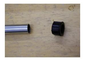
Photo 8: Silicone top cap and top end of outer siphon tube
