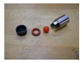
Photo 1: Check valve parts: bottom cap, o-ring, ball, body
