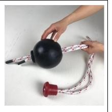
Stagger the rope ends to allow one to pass through at a time from the bottom flat plug
