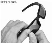
**3.** Work your way around the edges until all four corners of the lens are firmly snapped into the frame.
