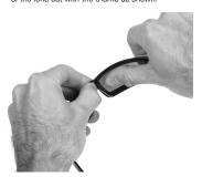
**3.** Using your thumb, push the lens out of its groove from the back.
