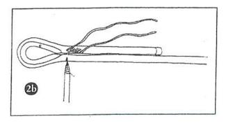
2b. For a thimble eye, allow a little space below the thimble. This will make it easier to finish the splice, and then if necessary you can seize the thimble in snugly. After marking, remove the thimble. You'll install it during Step #21. For "keeper thimble" installation, see Step #8.
