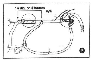
9. Pull as much core out of the rope as you readily can. This will bunch up the cover, making more room inside the rope for the tuck. Keep the cover bunched up as you tuck.
