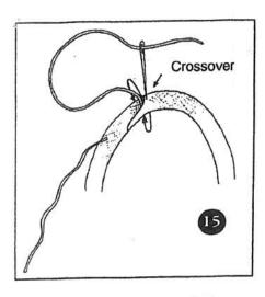
15. Using the second marker yarn, stitch the Crossover to make it secure and more compact. Pull the yarn home gently for the first 2 or 3 stitches, to avoid distorting the cover braid. Make subsequent stitches at varying angles, and seat them firmly.
