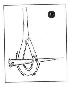
20. Watch the eye as the cover advances. If the eye starts to bunch up, stop immediately to get the slack out of the eye:
