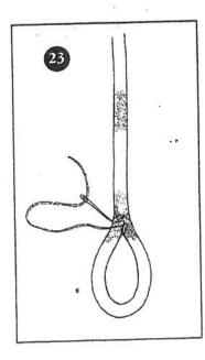
23. Use the marker yarn to stitch the splice, locking it in place to keep it from sliding apart under low loads (under high loads, the splice compresses on itself, precluding slippage).
