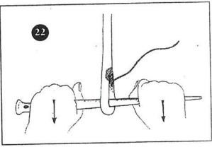
22. Pull on the eye with the spike and the cover should unbunch. If it doesn't, try a snapping motion to get it to move. If it still won't move, you may have waited too long to deal with the bunch. If this has happened, you'll need to pull a little core back out of the standing part, and try again. In the future, deal with this bunching as soon as you see it happening.
