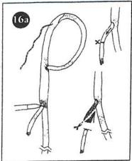
16a. Mark the core right where it exits. Pull out extra core.
