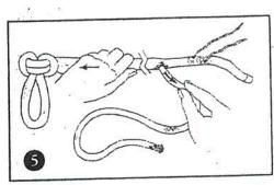
5. The next step is to "balance" the rope. This is an important step for any core-and-cover splice, as it assures that the core and cover will be under even tension.
