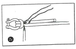
2c. For a Ring-Hitched eye, snug the hitch firmly before marking. After marking, remove the shackle. You'll hitch it back on after the splice is done.
