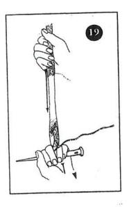
19. Keeping tension on the eye, start at the knot and firmly smooth the cover towards the eye. Depending on how far away the knot is, this could be a 2-person job.
