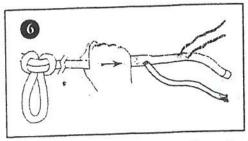
Slight differences in tension between the core and cover are not significant over the length of a rope, but an imbalance in the part that you are splicing could throw off the reference points (marks, marker yarns) that make the splice work. With one hand, hold the rope near where the core emerges. With the other hand, pull as much core out as you readily can. This will bunch up the cover.
