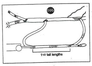
10b. If you are using a Splicing Wand, enter it into the core about 11/2 cover tail lengths on the standing part side of the prominent core mark. Bring it out at the mark.
