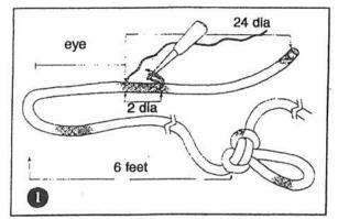
1. Pull out a single marker yarn, 24 diameters from the end. Pull out another single marker yarn about 2 diameters towards the end from the first. The first yarn marks one side of the eye. The second yarn marks where the core will enter the cover. Tie a Loop Knot about 6' beyond the eye.
