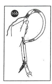
16b. Once again, firmly smooth the cover, as in step 14. This time, the core will disappear into the rope.
