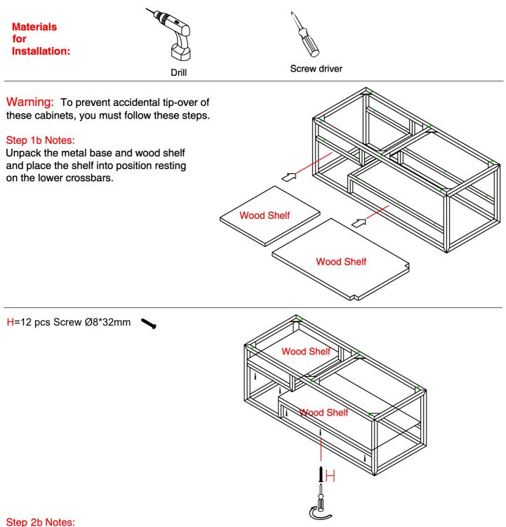
Insert and secure the screws (H) from underneath the metal base using a screw driver or an electric drill.
