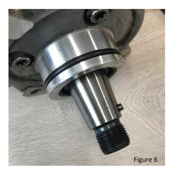
Once all o-rings and barrel and plunger assemblies are installed you are ready to re-install the pump.
