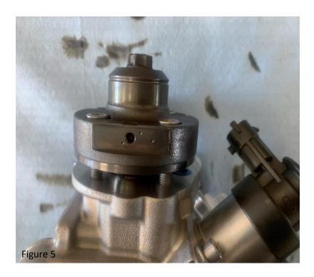
Slowly bring the barrel hat down by running the bolts in evenly together, once bolts are in, we recommend torqueing bolts to 108 inch/lbs or 9ft/lbs.
