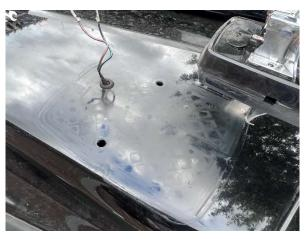
7. Place the Turn Signal Protection Guard Assembly onto the Hood Panel such that the two holes in the Base Plate(B) align with the holes in the Hood Panel and the Wires can be fed through the slot of the Base Plate.
