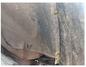
4. Reaching inside the Wheel Well Liner, remove the Nuts and Washers from the Turn Signal Housing Bolts and then remove the Turn Signal Housing Bolts from the Turn Signal Housing.
