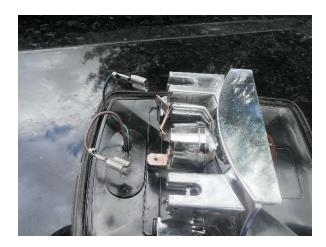
6. Remove the Turn Signal Seal and Turn Signal Housing carefully assuring the Wires are not damaged and then clean off the surface of the Hood Panel where the Turn Signal rests.
