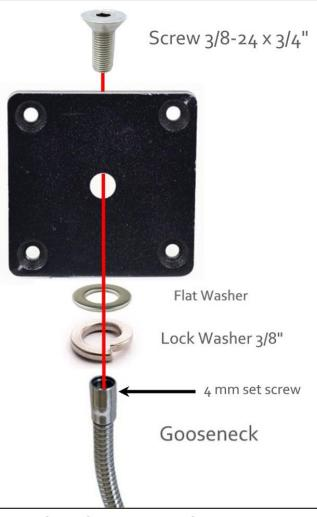
NOTE: Prior to inserting the 3/8" screw, you must first loosen the 4mm set screw. After tightening the 3/8" screw, GENTLY tighten the set screw.
