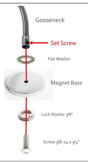
WARNING: Prior to inserting the 3/8" screw, you must first loosen the 4mm set screw. After tightening the 3/8" screw, GENTLY tighten the set screw.
