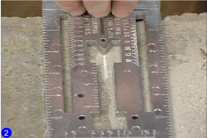
Line up center of tool with center mark.
