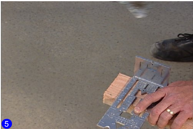
Place circular saw against the Universal Square and make a straight cut.
