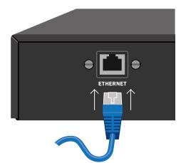
Connect a user supplied Ethernet cable to the rear of the Power Analyzer box connecting the other end to the user supplied network with internet access. For WiFi installations please refer to the Wifigurator Network Connection Guide for connection instructions.
