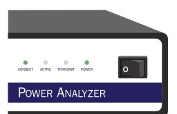
Make sure the 3-core power cable is properly connected to the rear of the Power Analyzer and the plug is connected to 110-270V AC power or 24V DC power as selected during installation. Turn the rocker power switch to the 'ON' position. Immediately, the LEDs corresponding to 'Power' will light. After approximately 30 seconds, the 'Connect' and 'Active' lights will turn on. If not, check power connections from the back of the Power Analyzer box to the supplied power.
