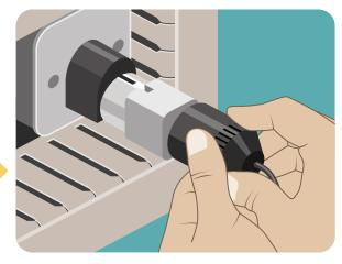
**NOTE**: The 3-core power cable will be connected to the 3-pin brass connector on the rear of the Power Analyzer Unit upon shipment.
