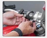
2. Select a location for the Bar Mount. Rotate the Arm and Head to desired angle, tighten Arm in place. Then, tighten Handlebar Clamp.
