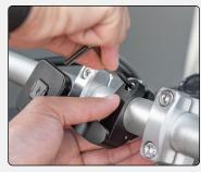
4. Lastly, tighten the Handlebar Clamp Screw to secure the mount in place.
