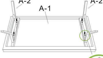
Don't tighten all screws until assembled complet
