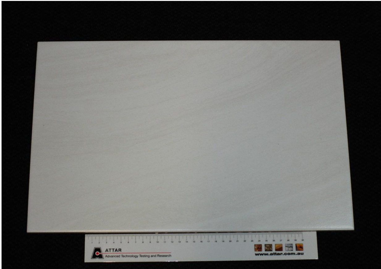
Figure 1: Porcelain tile with DuraGrip Plus HP-300 + Performance plus + 500 Grams of GripLok standard applied
