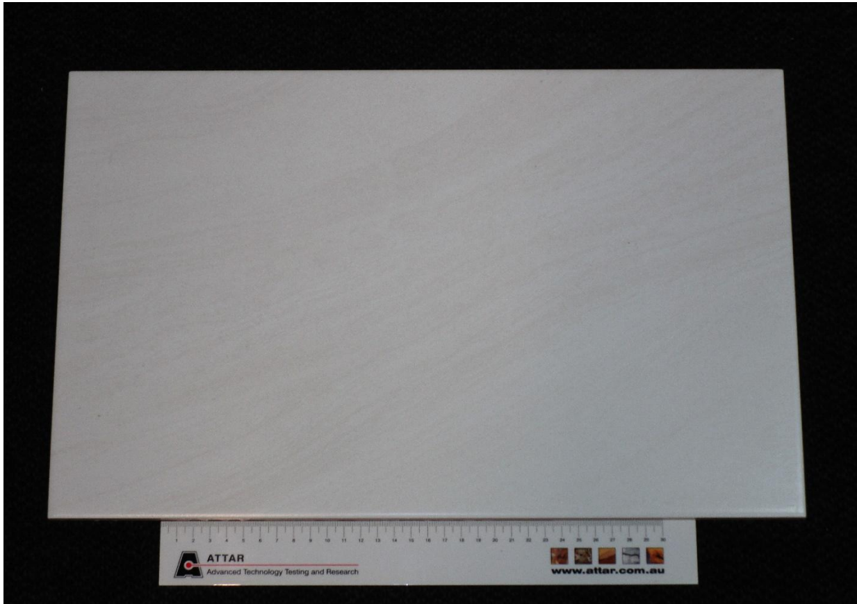
Figure 1: Porcelain tile with Satin DuraGrip PLUS HP-300 + Performance plus + 250 Grams of GripLok standard applied
