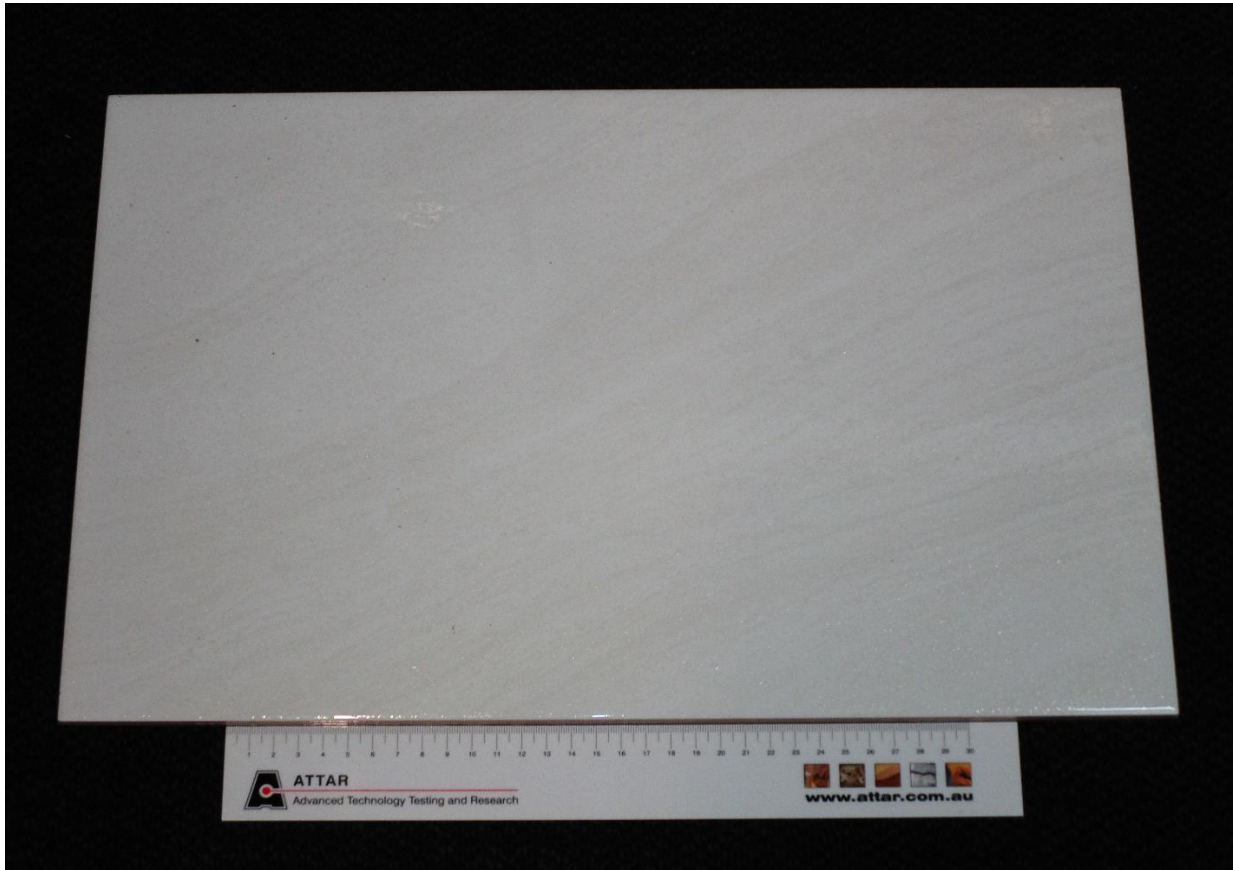
Figure 1: Porcelain tile with Gloss DuraGrip Plus HP-300 + Performance plus + 40 grams of GripLok Gloss applied.
