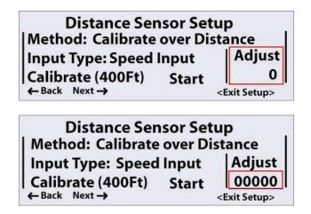
To manually adjust your speed constant, press the Adjust feature and a box will appear just around the numbers rotate the dial clockwise or counter clockwise to the desire number and then press enter. To manually adjust the speed that your monitor is displaying, go to the main screen to the feature Speed + or Speed – and adjust your speed to what you know it is. See page 8 and 9 for more details. This function will change your speed constant number corresponds to your speed adjustment.
